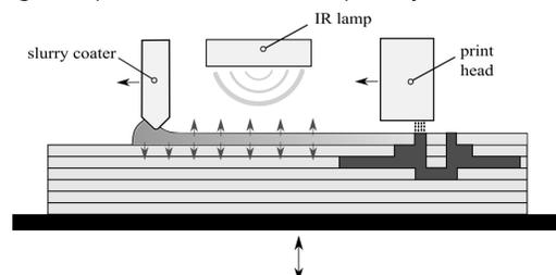
Figure 2: Schematic representation of the slurry-based binder jetting process [1]
