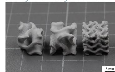
Figure 5: Demonstrators in the form of gyroids; from left to right: gyroid with a wall thickness of 1.5 mm; gyroid with a wall thickness of 2 mm; gyroid with a wall thickness of 1 mm.
