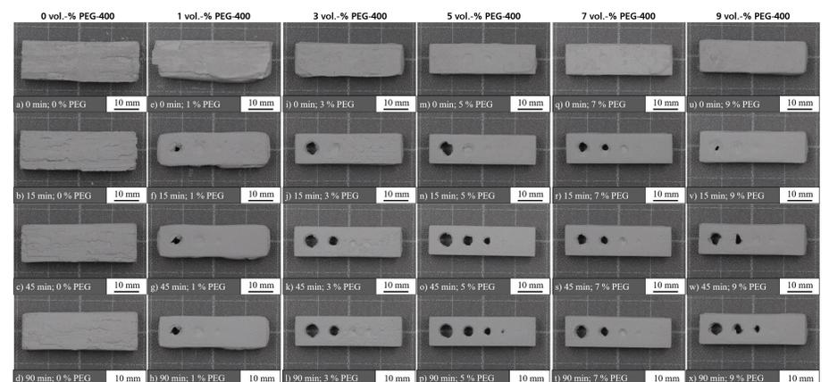
Figure 4: Wash-out process of green bodies at varying PEG-400 concentrations (0 vol.-%, 1 vol.-%, 3 vol.-%, 5 vol.-%, 7 vol.-%, and 9 vol.-%) over time (0 min, 15 min, 45 min, and 90 min). The panel with 5 vol.-% PEG-400 (pictures m through p) demonstrate the best wash-out results, showing 4 free through holes after 90 min (picture e).
