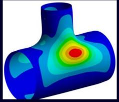
Geometry leads to inhomogeneous stress in the part
