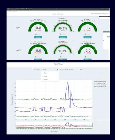
Generate and visualize the digital fingerprint based on synchronized high frequency data from process sensors on an edge device Currently for SINUMERIK driven machines
