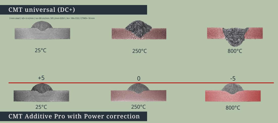
3 mm steel / vD= 6 m/min / vs= 80 cm/min / Ø1,2mm G3Si1 / Ar+ 5% CO2 / CTWD= 18 mm
