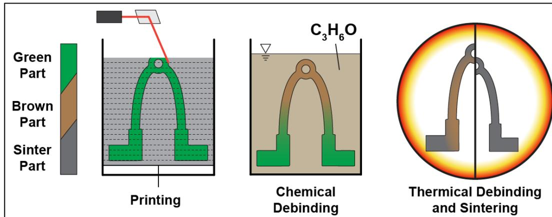
Fig.: Process steps of Cold Metal Fusion
