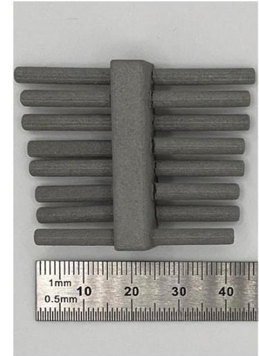
Fig.: Close up of exemplary CMF-specimen after sintering
