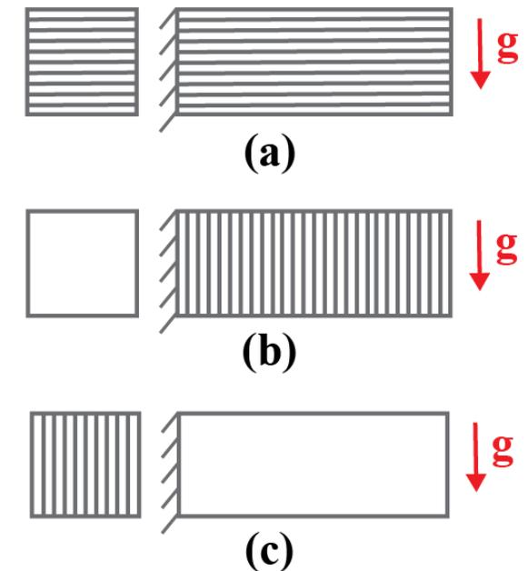
Fig.: Build orientation set-ups for MFFF-specimens
