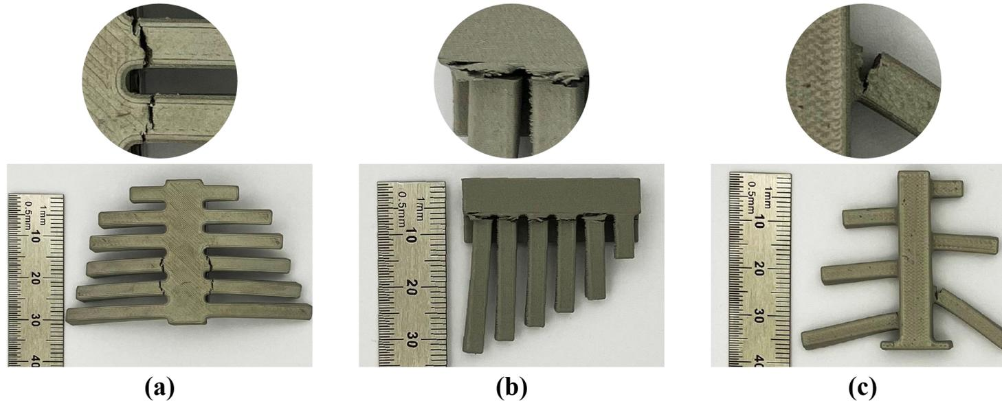
Fig.: MFFF-specimens with close up of fractures
