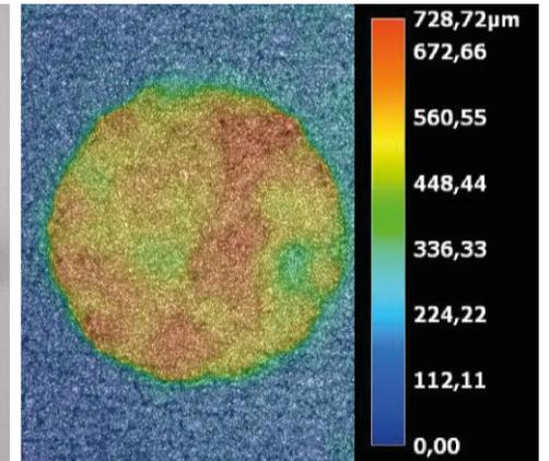
Fig.: CMF-specimen and fracture surface with elevation profile
