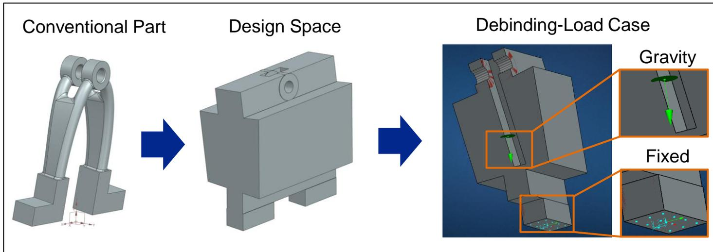
Fig.: Workflow for topology optimization
