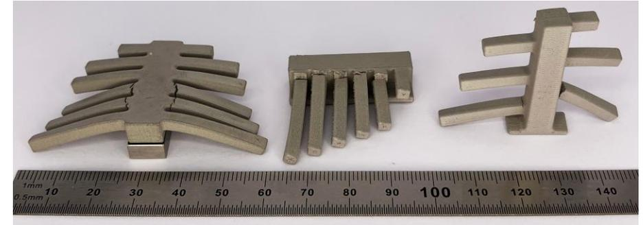
Fig.: MFFF-specimens in perspective
