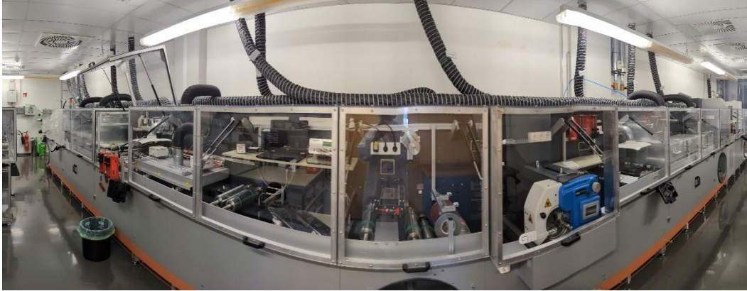
Roll to Roll printing, 3 Stations, 13 m Ovens, Screen printer Inline on-the-fly laser
