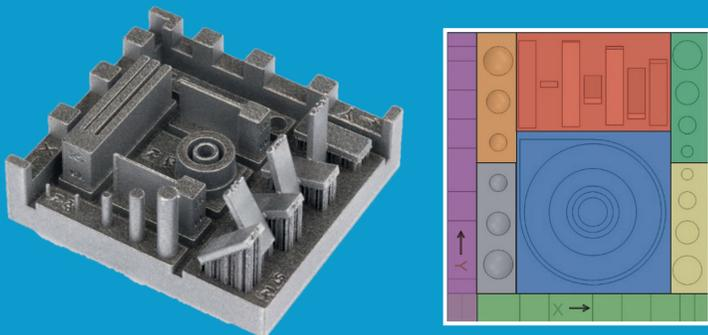
Figure 1: Test artefact according to DIN EN ISO/ASTM 52902
